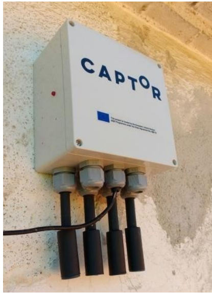
CAPTOR: metal oxide low-cost sensors (UPC)
