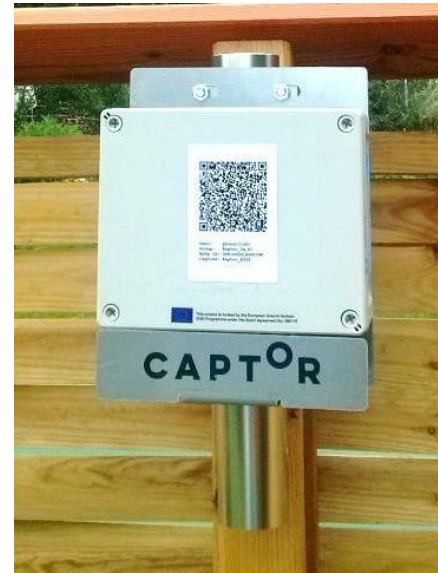
RAPTOR: electrochemical low-cost sensors (UCA)
